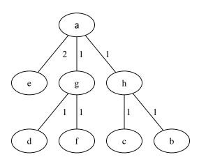
We get the cycle  $a \to e \to a \to g \to d \to g \to f \to g \to a \to h \to c \to b \to h \to a$ , in which every point is visited at least once (indeed, a number of times equal to its degree in the tree) and every edge is traversed precisely twice.
