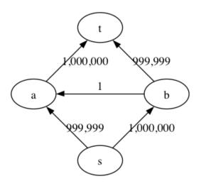
Now it is possible that the algorithm picks the augmenting path  $s \to b \to a \to t$  along which, again, only one unit of flow can be routed. We see that, indeed, it is possible for the algorithm to keep picking augmenting paths that involve a link between a and b, so that only one extra unit of flow is routed at each step.
