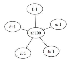
Then the algorithm would start from the edge (a, b), and cover it by putting a, b into S. This would suffice to cover all edges, but would have cost 101, which is much worse than the optimal solution which consists in picking the vertices  $\{b, c, d, e, f\}$ , with a cost of 5.
