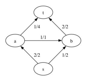
Is the flow optimal? We are only sending 3 units of flow from s to t, while we see that we can send 2 units along the  $s \to a \to t$  path, and another 2 units along the  $s \to b \to t$  path,
