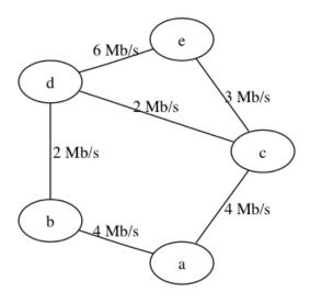
The answer is yes: a can split its stream of data, and send 4Mb/s to c and 2Mb/s to b. The node b relays the 2Mb/s stream of data that it receives from a to d, while node c splits the 4Mb/s stream that it receives into two parts: it relays 3Mb/s of data to e, and send the remaining 1Mb/s to d. Overall, d receives 3Mb/s of data, which it relays to e.
